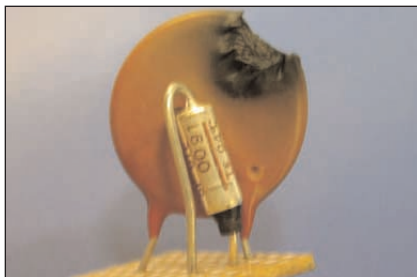
Figure 6b. MOV/TCO combination
