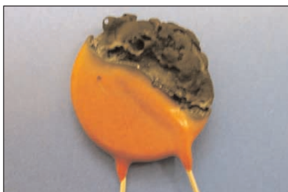
Figure 6a. Standard MOV
