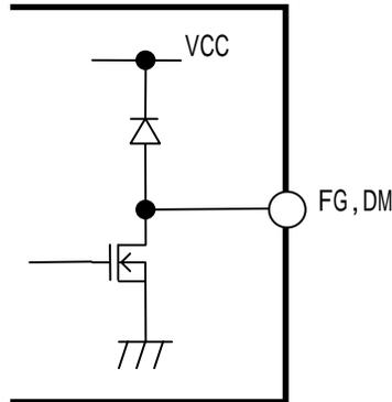
Figure 4. Equivalent circuit around FG, DM terminals
