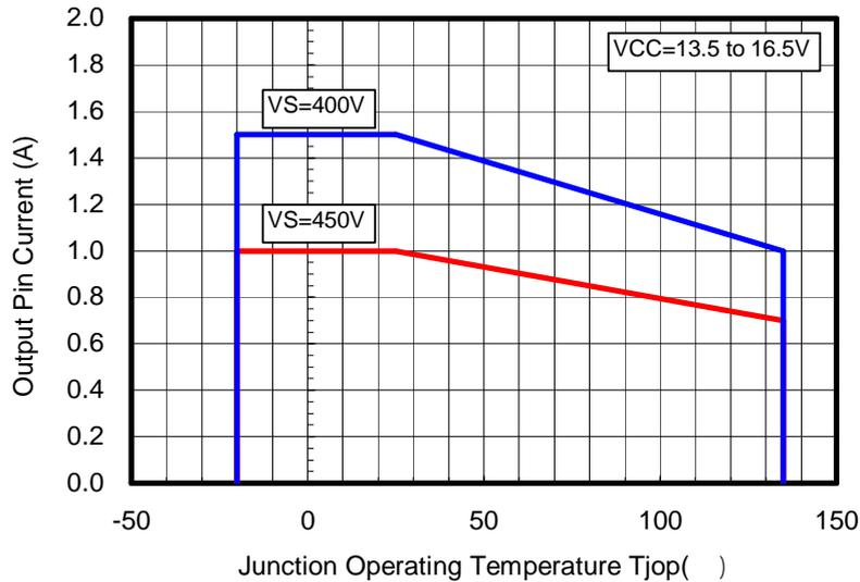
Figure 9. Current Derating for Junction Operating Temperature
