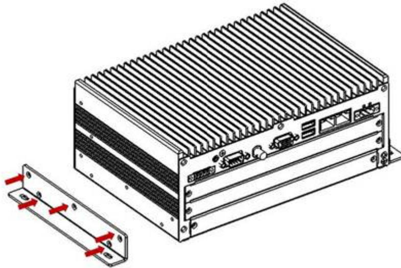
2. Use the 4 screw holes to mount the ECU-1871 on the wall.
