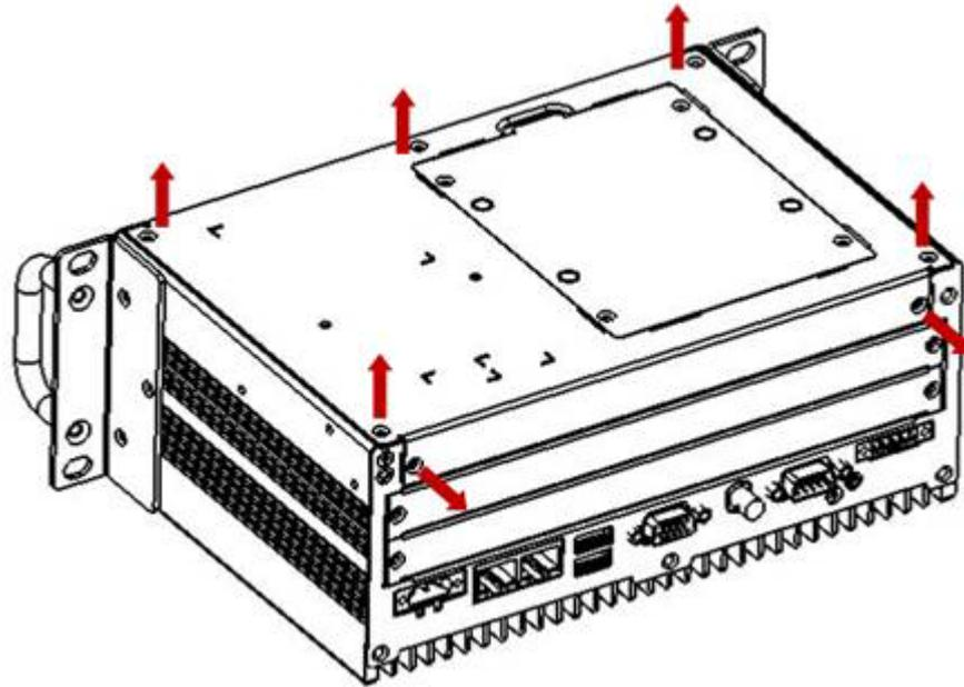
4. Remove the L-shaped cover (with HDD BRK)
