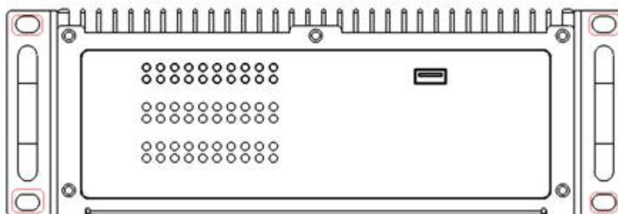
3. ECU-1871 equips the Aluminum Fins on the top of the unit as heat-sink. It can generate nature convection for better heat transmission. To have optimal thermal performance, please leave 2U (440 mm) space height on the top of the unit
