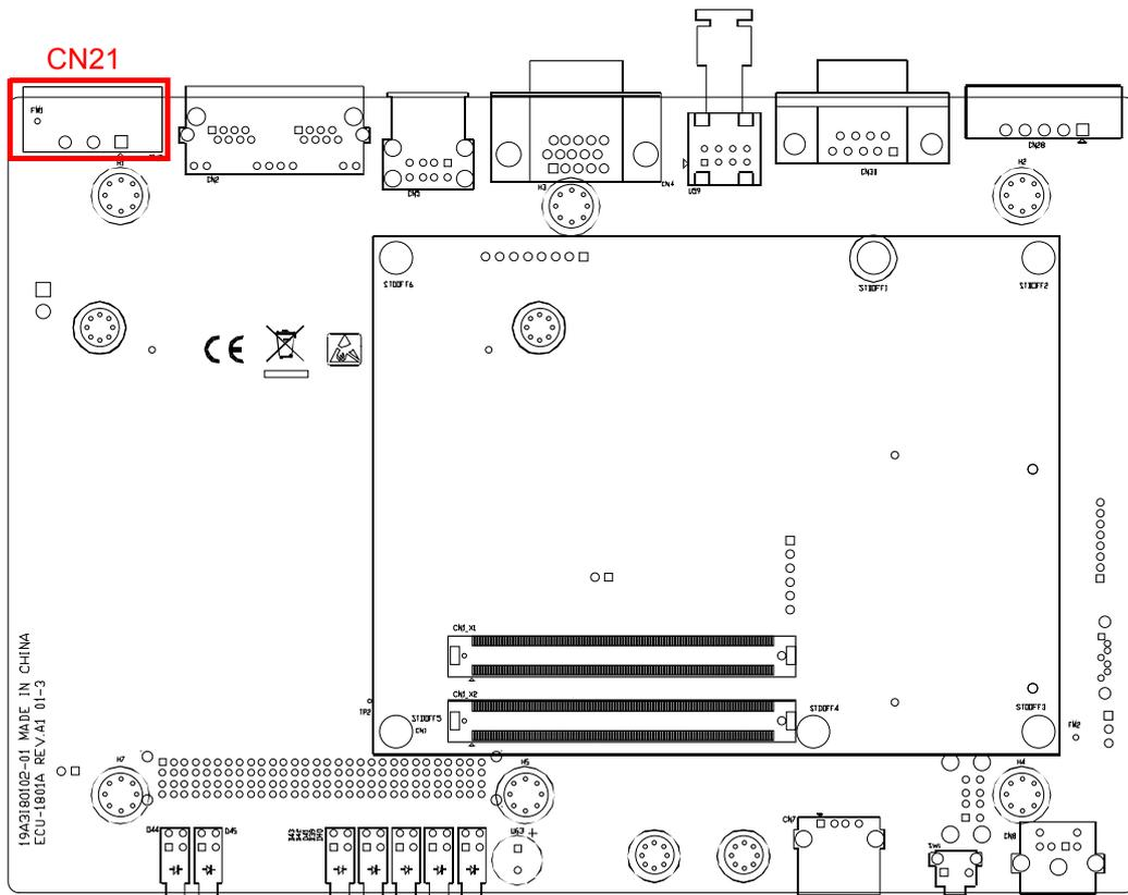
**Figure 2.4 Power input location(CN21)**
