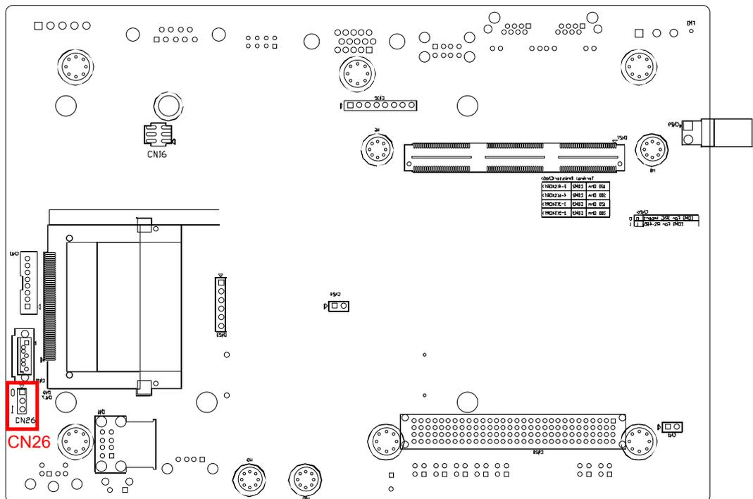
Figure 2.7 COM3 setting IRIG-B jumper location(CN26)
