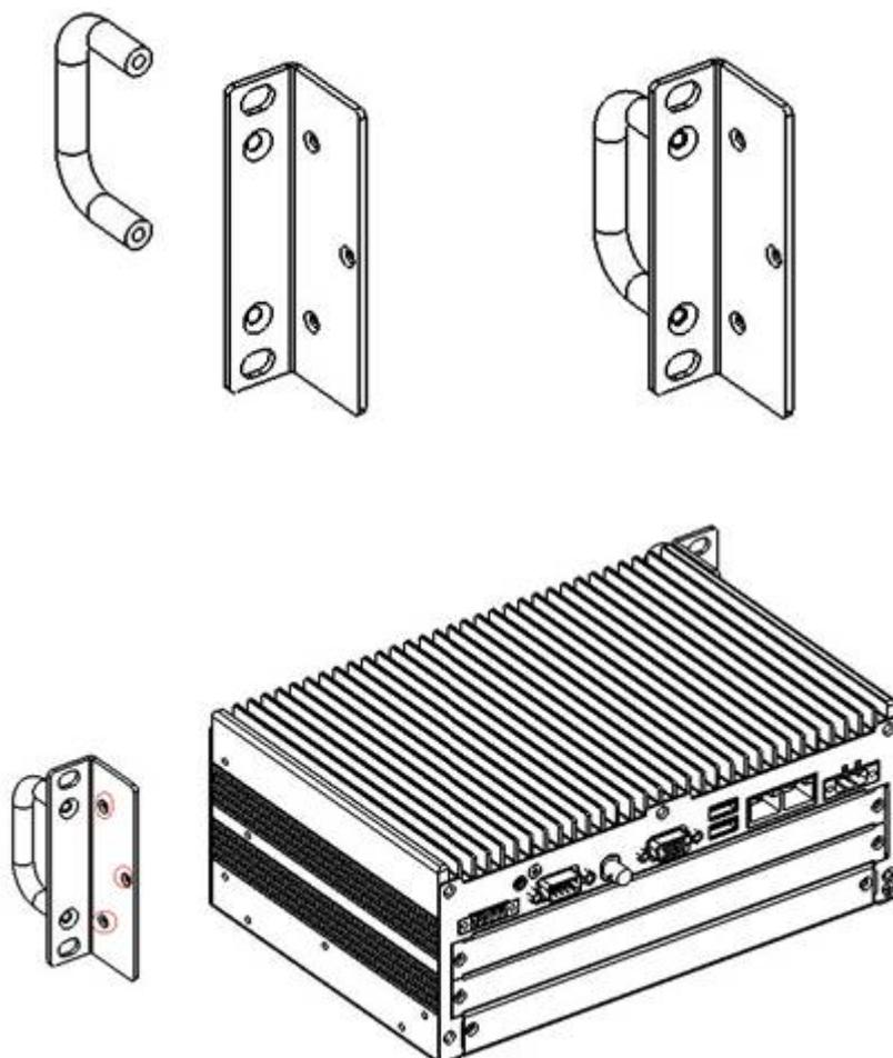
2. Use the 4 screw holes to mount the ECU-1871 on the rack.
