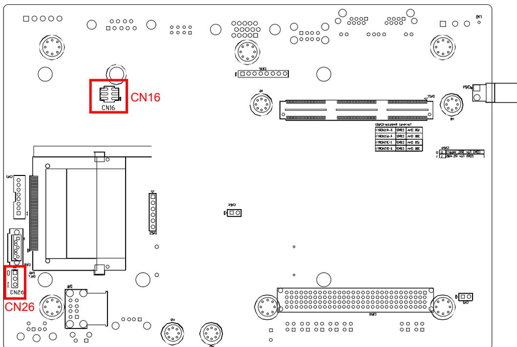
**Figure 2.3 CN16 CN26 position diagram**
