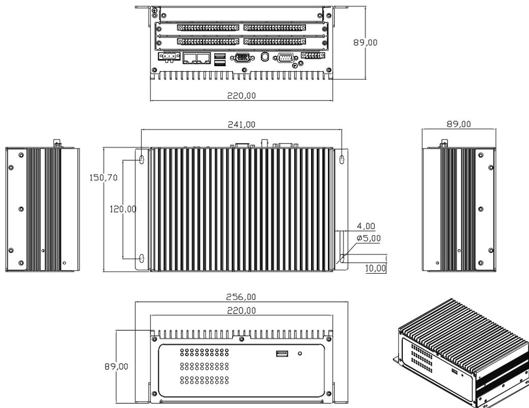
Figure 1.2 ECU-1871 Chassis Wall-mount mounting size
