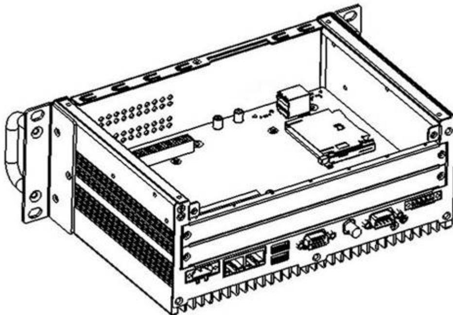
**Note!** *If an HDD is installed, please remove any HDD related connections before opening the chassis.*
