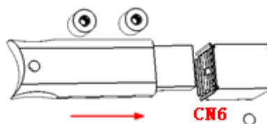
3. Adjust the position of the kit to fasten the USB dongle, and then screw to fix the kit.
