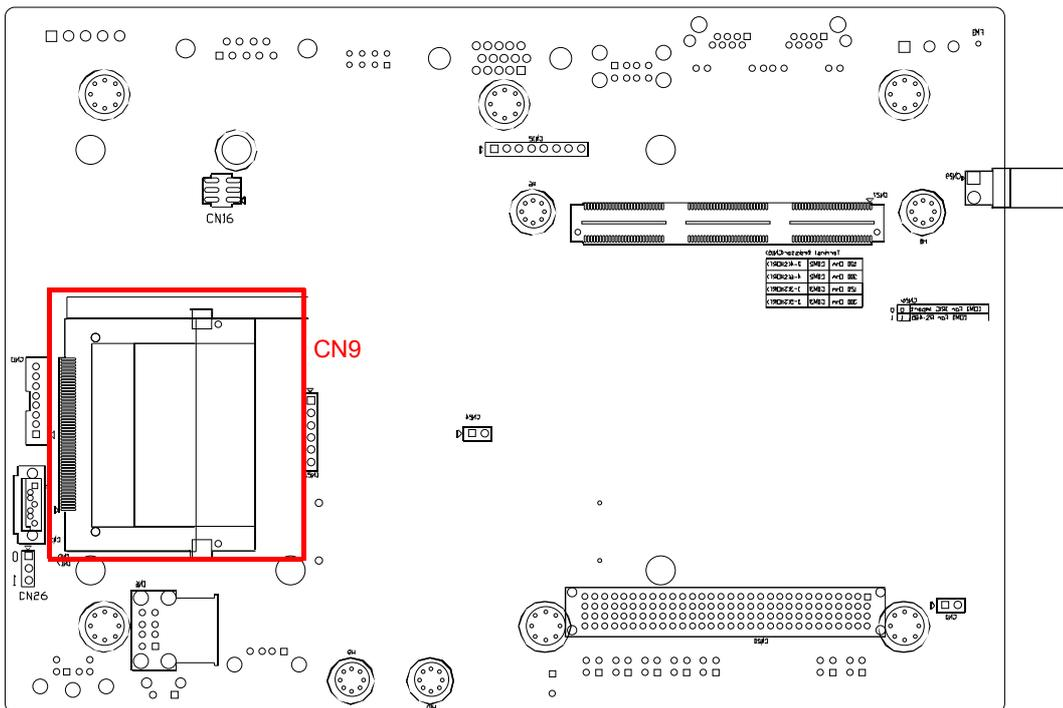
Figure 3.1 CompactFlash Card Slot Location(CN9)
