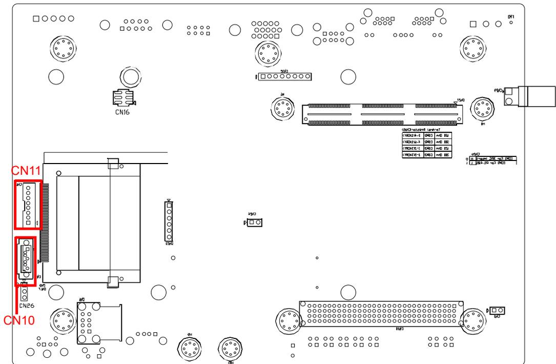
**Figure 3.3 SATA Signal and Power Connector Location(CN10 CN11)**
