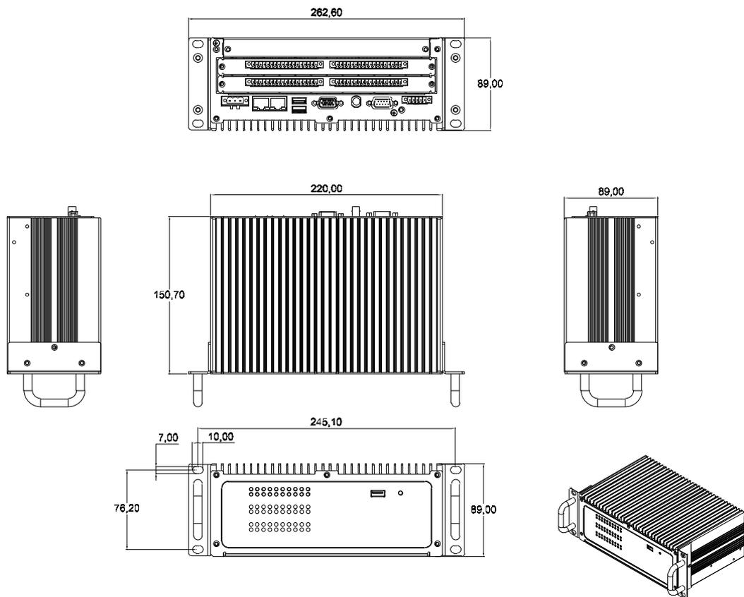
Figure 1.1 ECU-1871 Chassis Rack-mount mounting size
