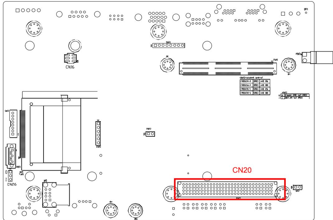
Figure 2.8 PCI-104(CN20) Location
