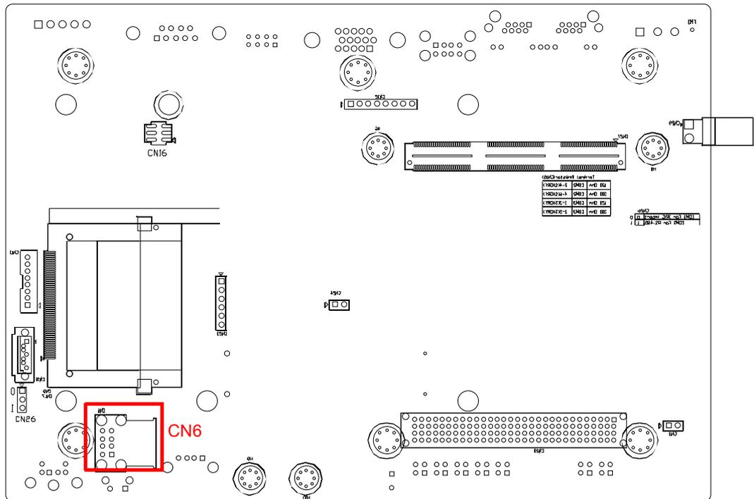
Figure 3.2 CN6 Location of Internal USB Port(CN6)
