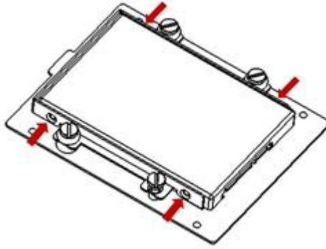
4. Connect the SATA cable between HDD and connector then assemble the HDD back to the chassis. The locations of the connectors are shown below, SATA signal connector locates on CN10 and SATA power connector locates on CN11.
