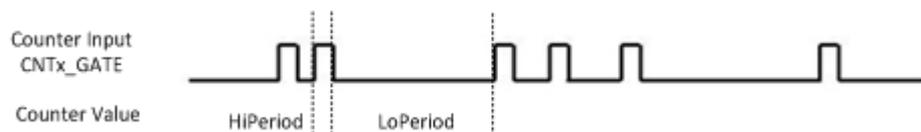
4. Pulse Output with Timer Interrupt: ECU-P1706 counter has internal clock that you can produce periodic output signal with interrupt generated at the same time. ECU-P1706 counter will use internal clock as time base, to fulfill the frequency you want to set. Available output frequency range is 0.005 Hz ~ 1 MHz.
