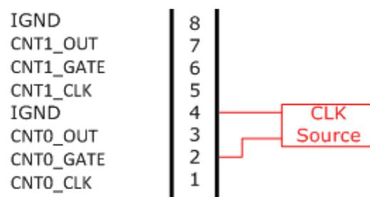
Figure 3.6 Frequency Measurement Connection
