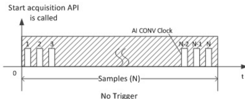
Set Trigger Source to None to enable this mode. The other 4 trigger parameters will be omitted by ECU-P1706 driver and take no effect in this mode.
