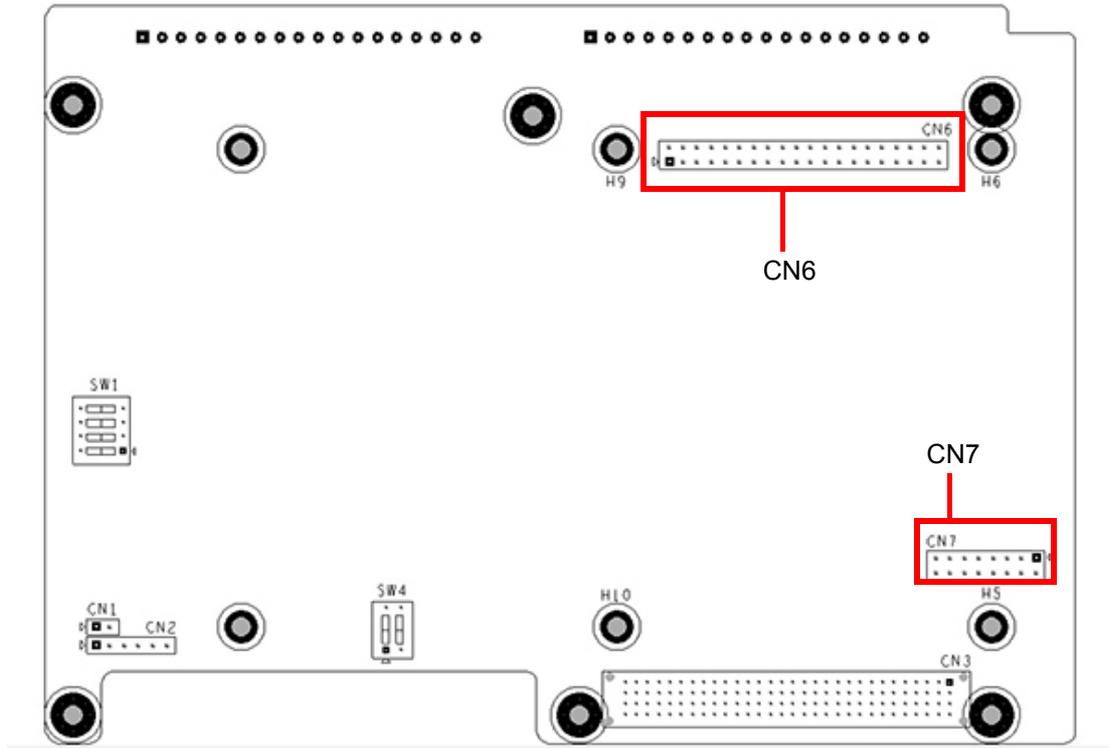
**Figure 2.4 Jumper (Extend connector) Location**
