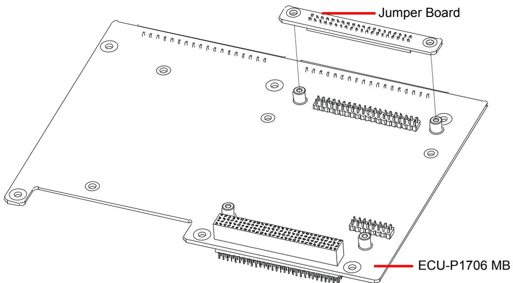
Figure 2.3 ECU-P1706-AE Exploded Diagram
