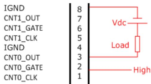
Figure 3.10 PwModulator Connection (PWM\_OUT)
