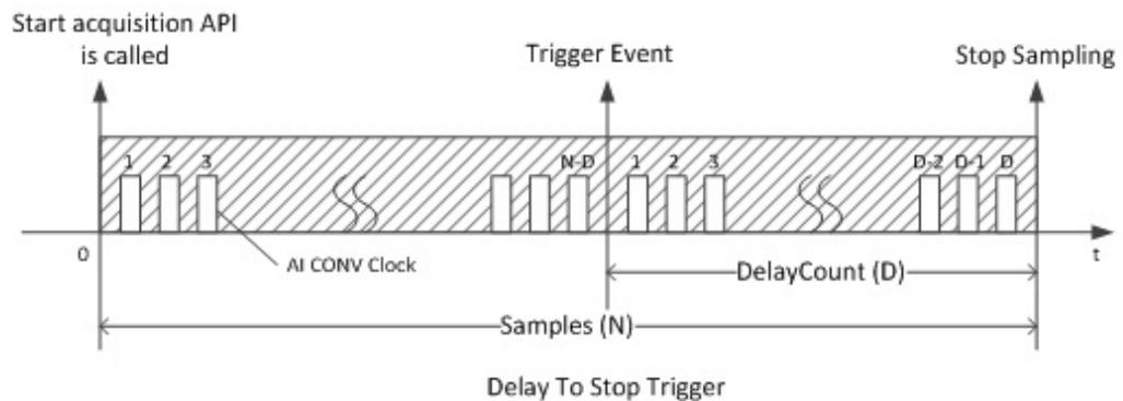
After the Trigger Delay Count (D), the process will stop automatically and returns the latest N samples, containing D samples after the trigger event and N-D samples before the trigger event.
