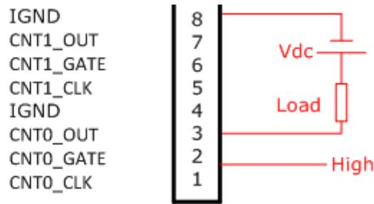
Figure 3.7 Time Pulse Connection
