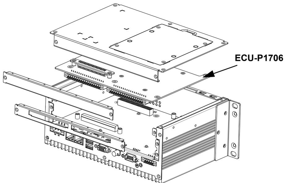
**Figure 2.5 ECU-1871 + ECU-P1706 Blasting Diagram**
