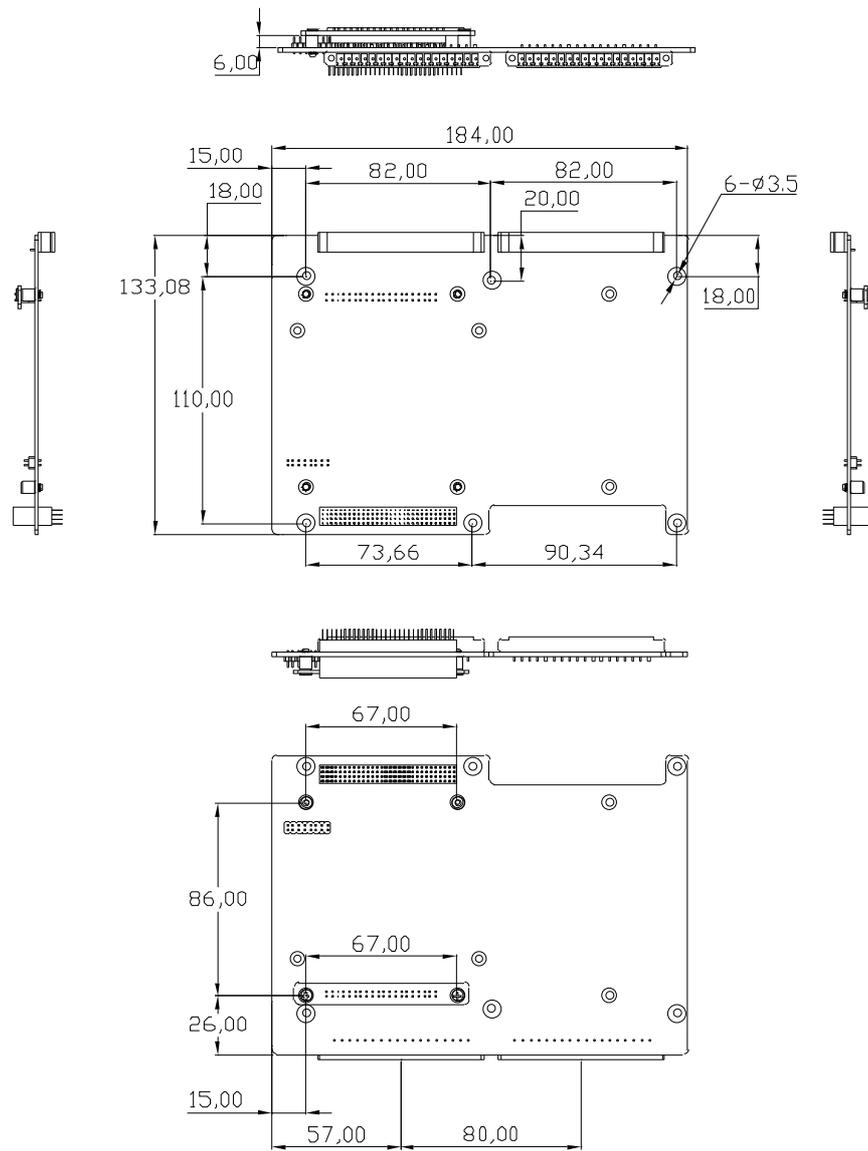
Figure 1.3 ECU-P1706 Dimensions Diagram
