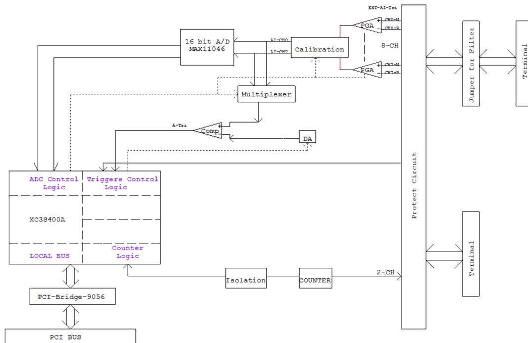
Figure 1.2 ECU-P1706 Function Block
