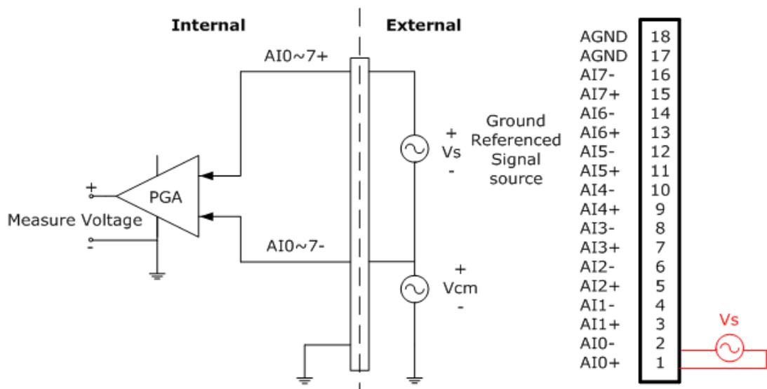
**Figure 3.3 Differential Input Channel Connection**
