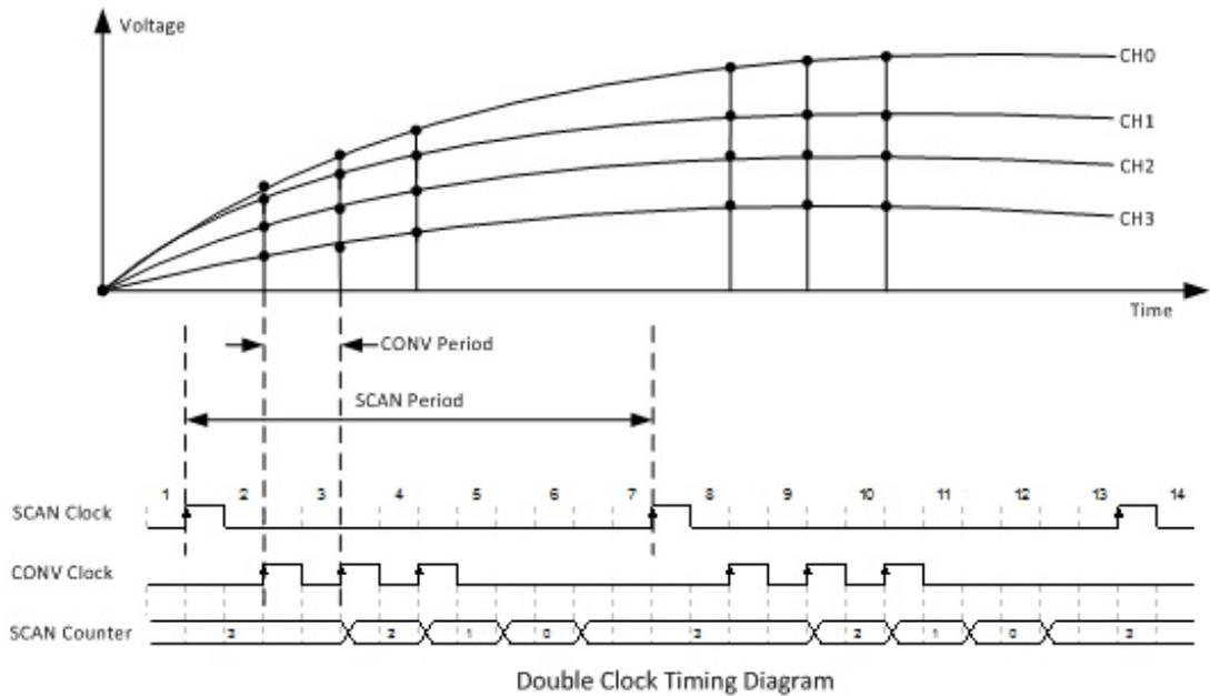
Once the acquisition procedure inside Acquisition Windows is set, the incoming CLKs must fit in the user-specified acquisition sequence, or the CLKs may be gated off. Refer to the following figures for more details.
