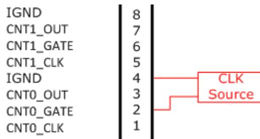
Figure 3.9 PwMeter Connection (PWM\_IN)
