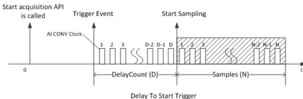
Delay To Start trigger mode is typically used when Trigger Delay Count (D) is set to 1 (the minimum), which immediately starts a simultaneous multi-channel acquisition when one of the channel's signal voltage reaches a specific value, such as 0V of a sine wave.
