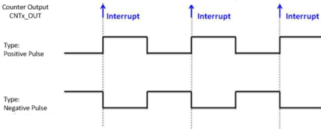
5. Delay Pulse Generation: Using ECU-P1706 internal clock, you can change the logic level within a specific period, starting from a trigger signal connecting to counter gate input. For example, if you define the count equals to 3 (as figure below), a counter output will change its status after 3 pulses of internal clock signals pass, after a trigger signal from counter gate becomes high.
