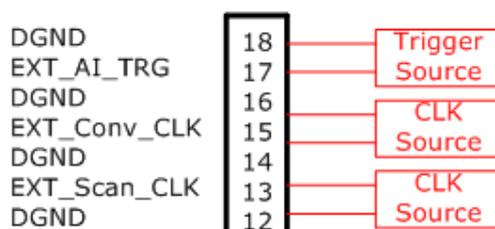
Figure 3.4 Trigger Source and CLK Source Connection
