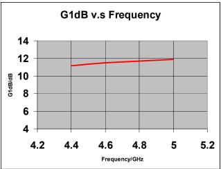
$V_{DS} = 10 \text{ V}, I_{DSQ} \approx 4500 \text{mA}$
