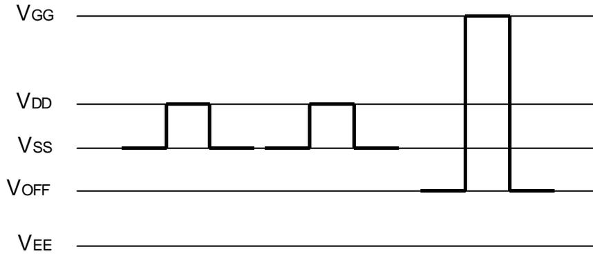
**Fig. 2.** Relative position of the different supply voltages
