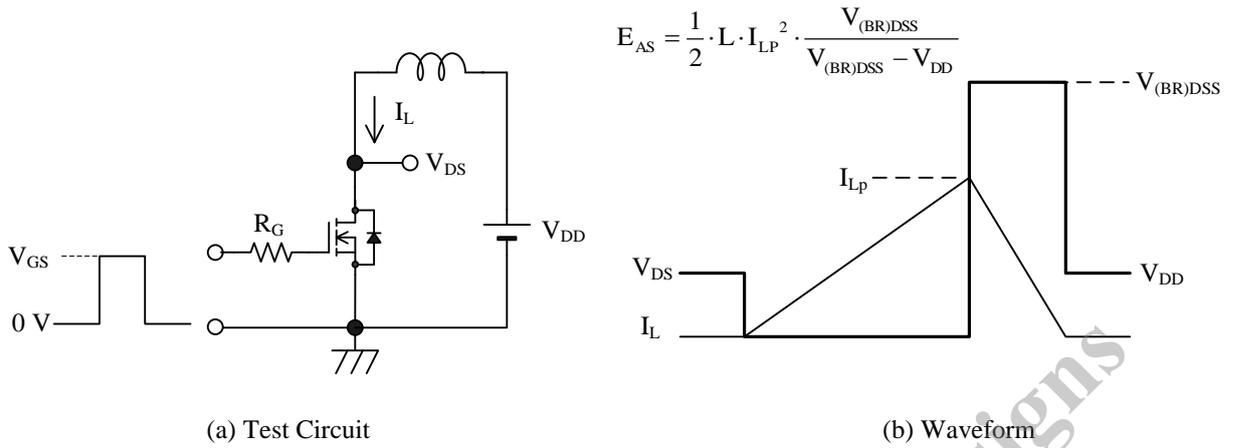
Figure 1. Unclamped Inductive
