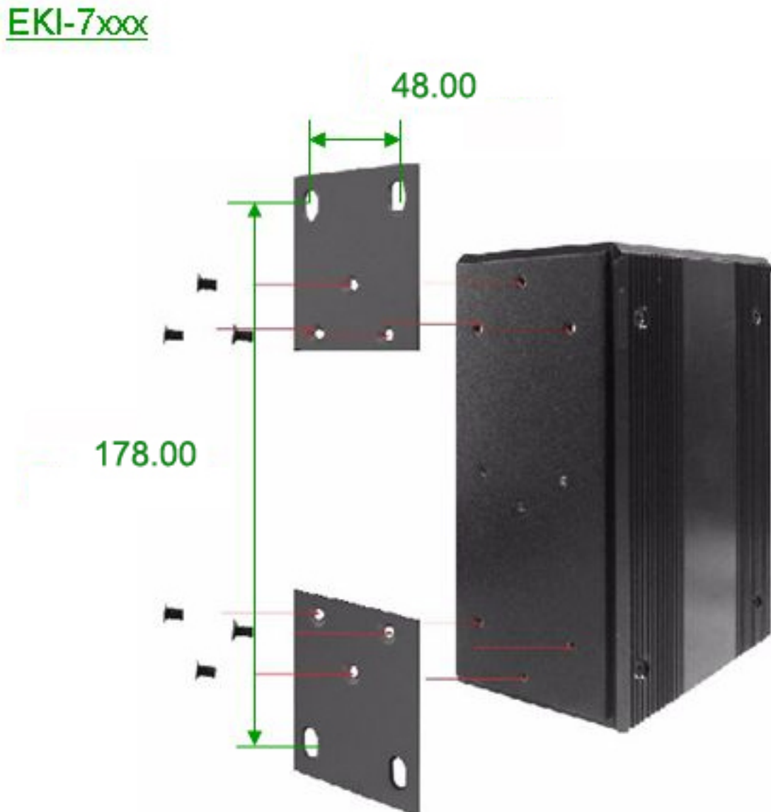
Figure 2.5: Combine the Metal Mounting Kit
