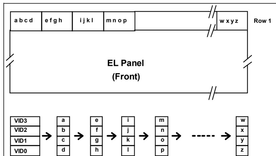
**Figure 3. Pixel Location versus Sequence of Data.**
