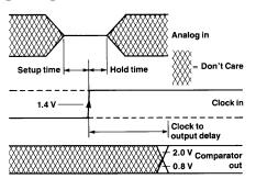
Note: Since the hold time is negative the input is a don't care at the clock time. This ensures that clock noise will not affect the measurement.
