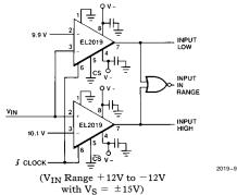
The EL2019 makes an excellent comparator in most analog to digital converters, due to its high gain and fast response. Most 2504 based A to D designs can be modified to use the EL2019 simply by using an inverted clock to the EL2019 as shown below. This results in improved performance due to less jitter of the transition voltages.
