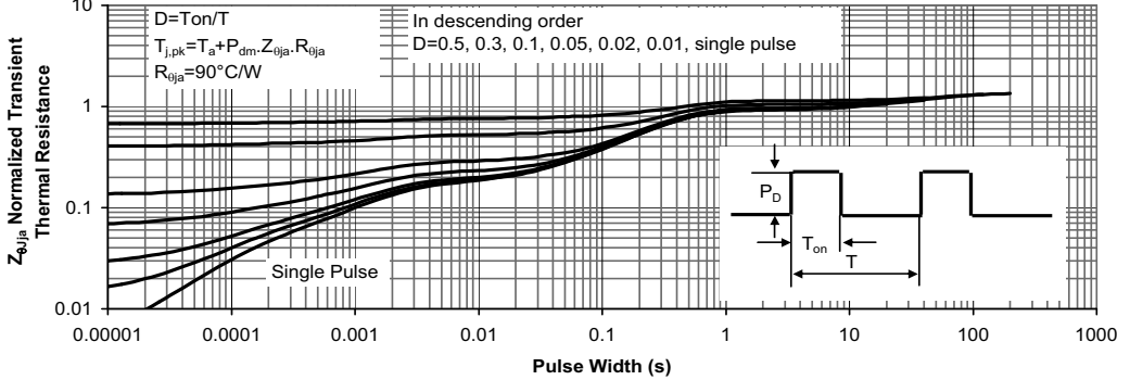
Figure 11: Normalized Maximum Transient Thermal Impedance
