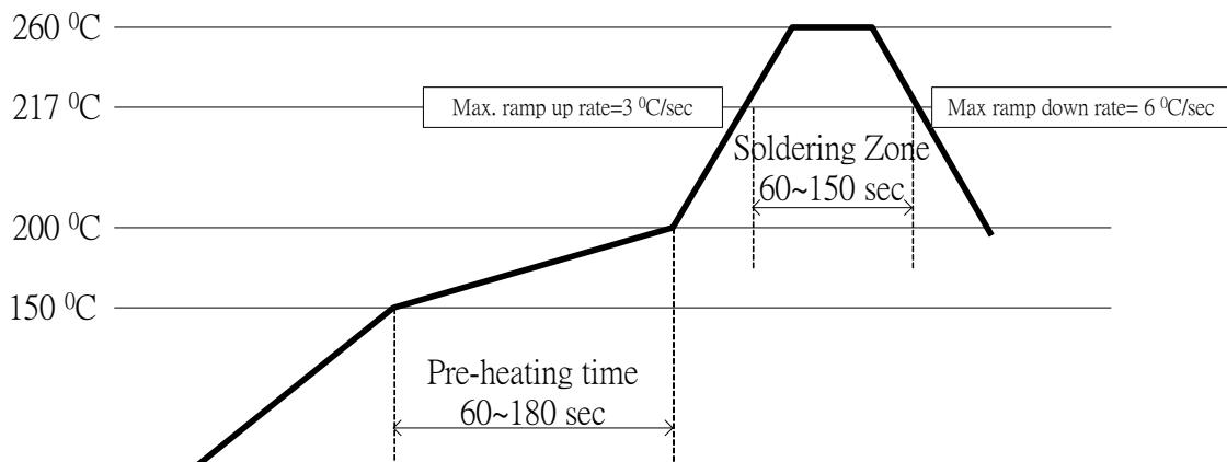
Note <sup>1</sup>: Reflow soldering should not be done more than three times
