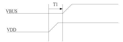
Note: The T1 time is recommended more than 30ms (VDD first is recommended)
