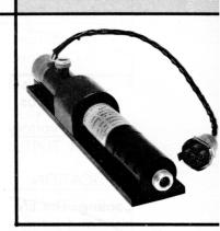
The EM-1011 features rugged ceramic and metal construction and focusing is provided by built-in periodic permanent magnets. These magnets are fully temperature compensated to allow operation from  $-55^{\circ}\text{C}$  to  $+85^{\circ}\text{C}$ . No additional cooling is required at these temperatures due to the integral heat sink/mounting flange supplied with the tube.
