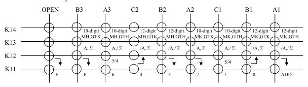
K14 : Select with Calculated Digits and Memory Hold Status, MH (Memory Hold), MK (Memory Kill), GTH(GT Memory Hold) and GTX(GT Memory Kill) at Auto Power OFF or OFF key.
