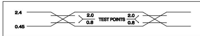
AC Testing: Input are driven at 2.4V for logic "1", and 0.45V for logic "0". Timing measurements are made at 2.0V for logic "1", and 0.8V for logic "0".
