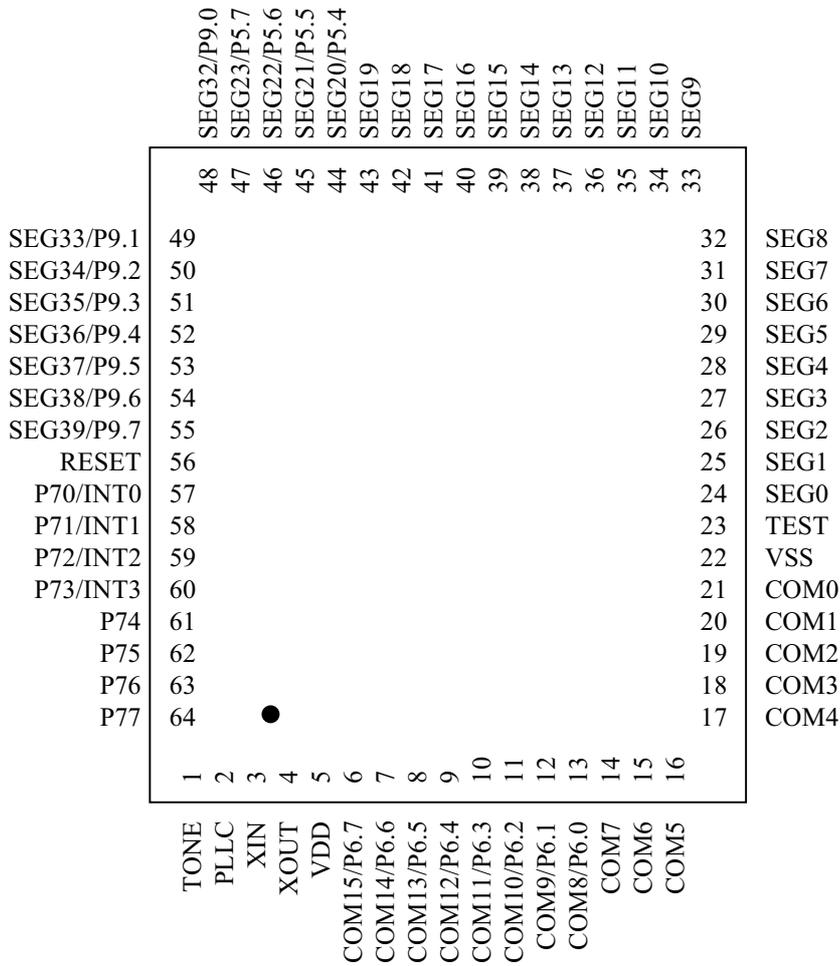
Fig.1 Pin Assignment
