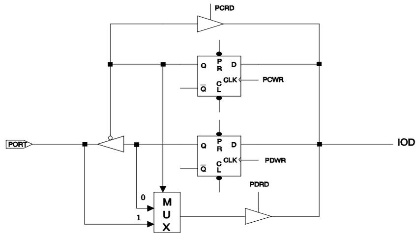
Fig.11 The circuit of I/O port and I/O control register
