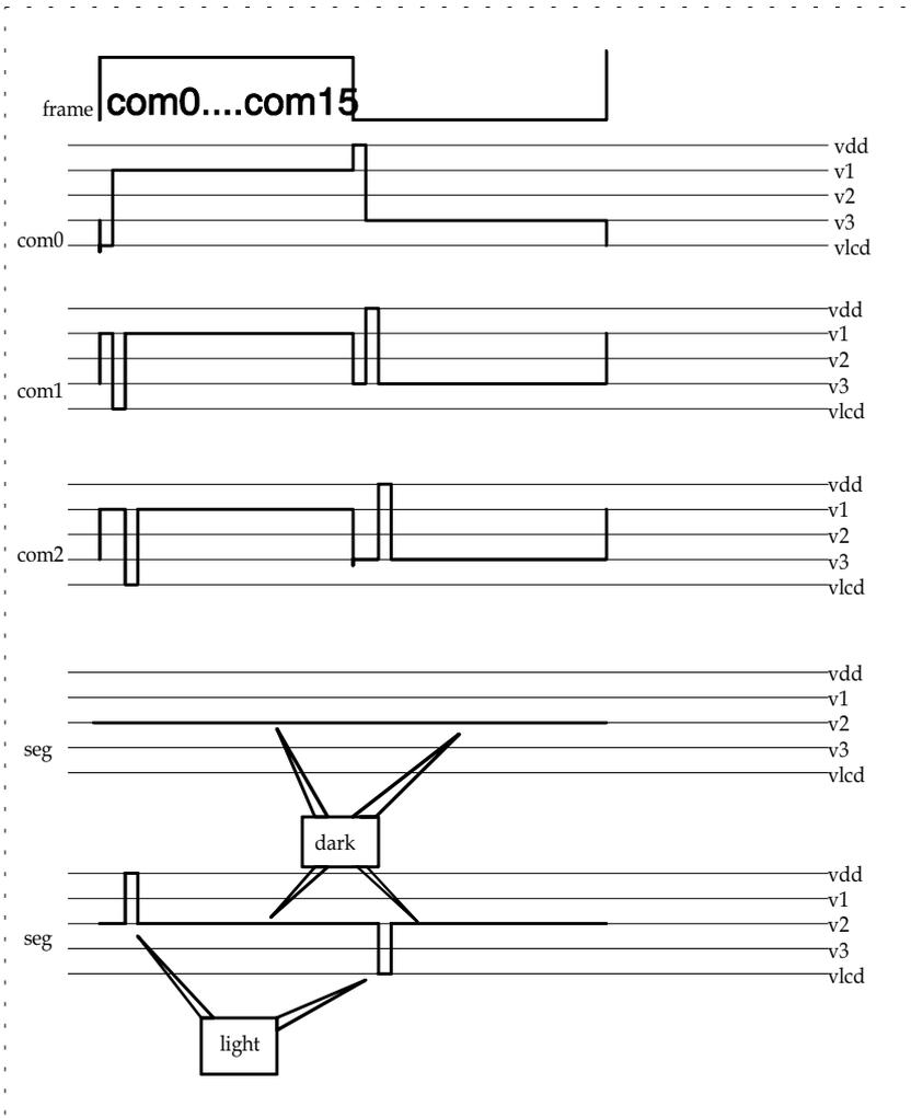
Fig.19 Lcd wave 1/4 bias , 1/16 duty
