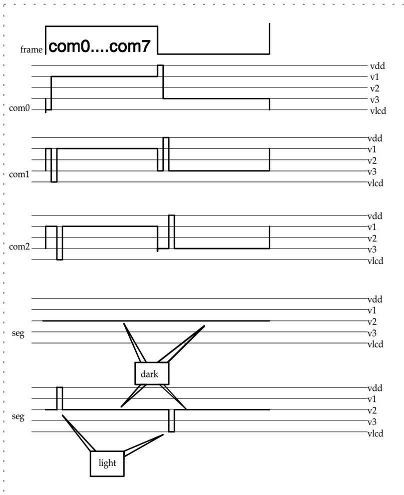
Fig.18 Lcd wave 1/4 bias , 1/8 duty
