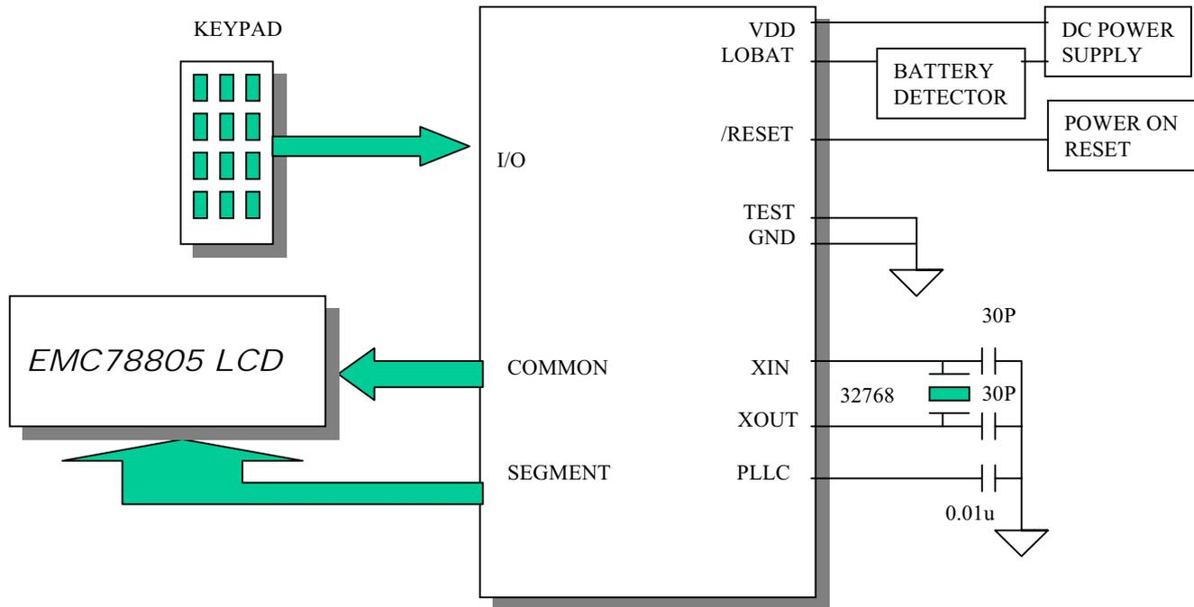
Fig.23 application circuit
