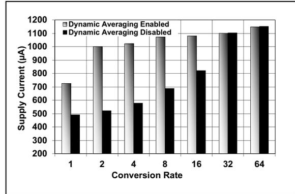
**FIGURE 2-7:** Supply Current vs. Conversion Rate.
