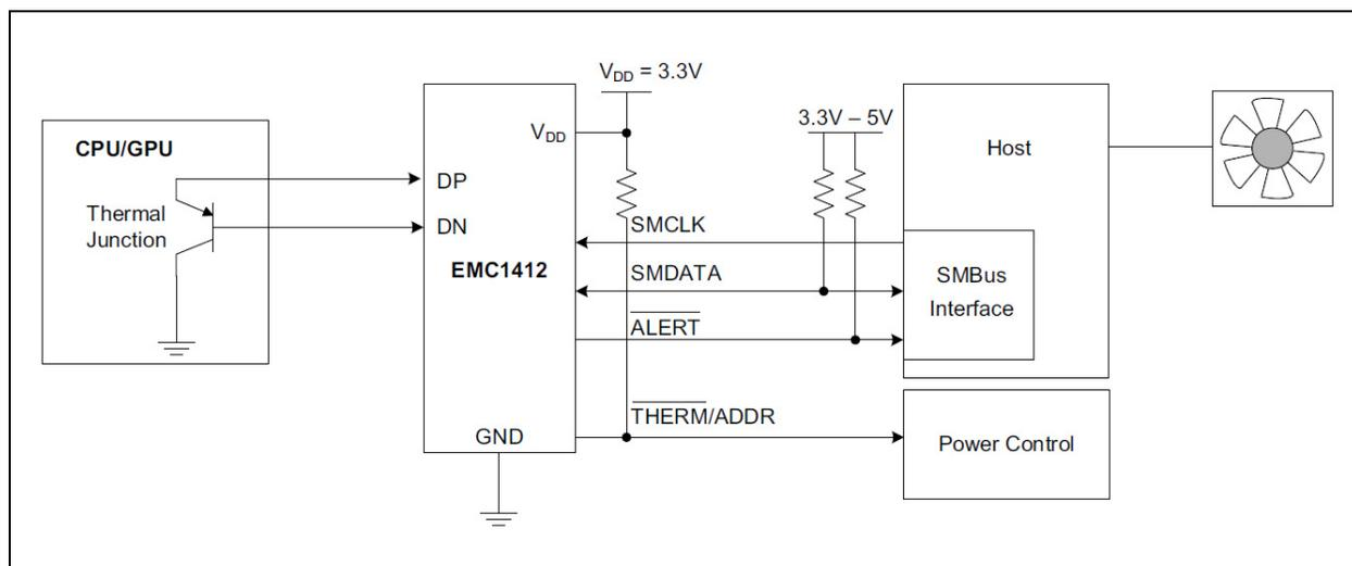
FIGURE 4-1: System Diagram.
