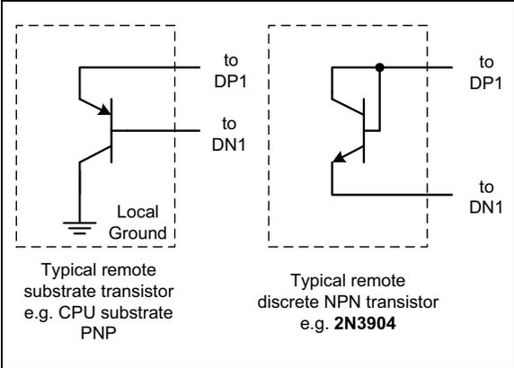
FIGURE 4-4: Diode Configuration.
