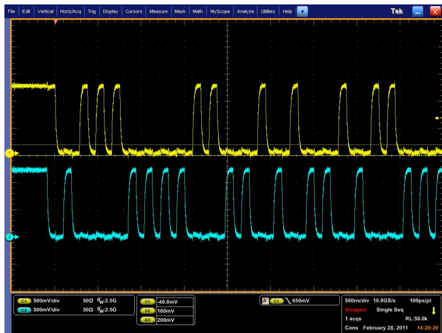
Figure 5. EMI4193 MIPI D-PHY LP Mode Measured Results
