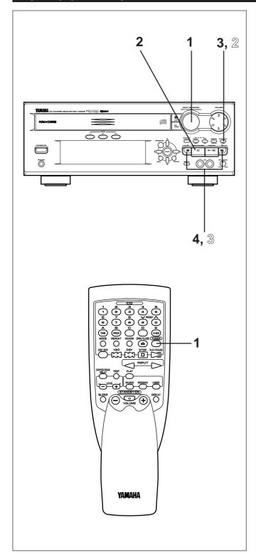
Normally, if station signals are strong and there is no interference, quick automatic-search tuning (Automatic tuning) is possible. However, if signals of the station you want to select are weak, you must tune to it manually (Manual tuning).
