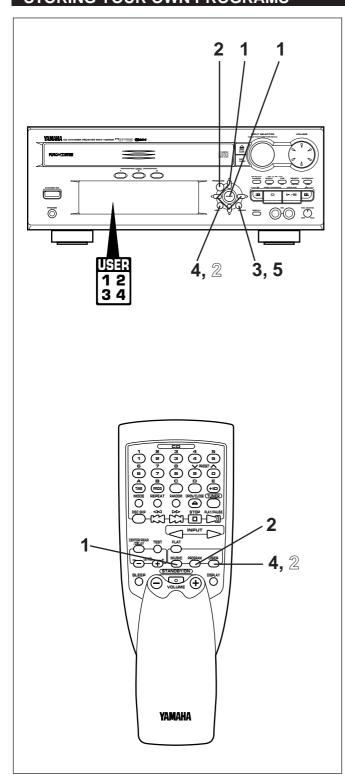
Your favorite pair of any equalizer mode (or an equalizer pattern of your own adjusting) and any sound field program can be stored as a user program. Up to 4 pairs can be stored as desired.
