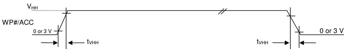
**Figure 12. Sector (Group) Protect and Chip Unprotect Timing Diagram**
