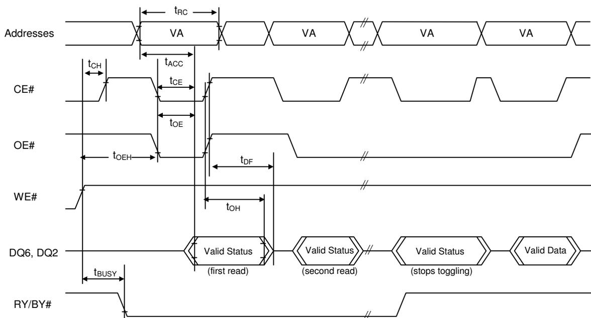
**Figure 8. Alternate CE# Controlled Write Operation Timings**
