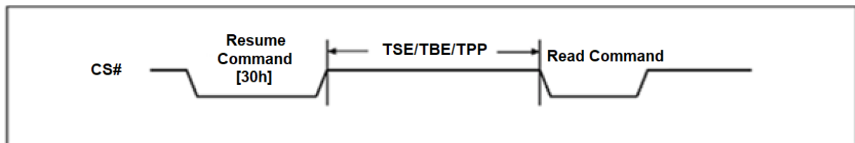
Figure 53. Resume to Read Latency
