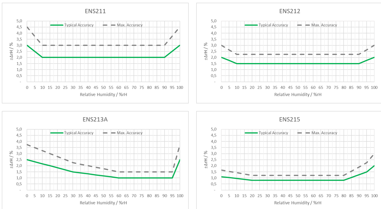
Figure 8: Relative humidity sensor accuracies 11
