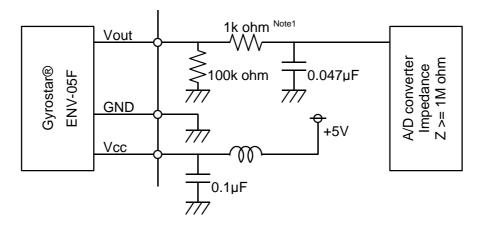
Note1) The value of this resistance should be 1/1000 or less of impedance of A/D converter
