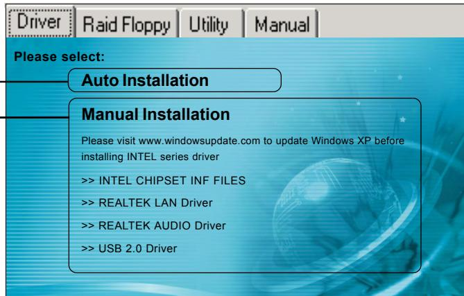
Insert the bundled CD into the CD-ROM and the main menu screen will appear. The main menu displays links to the supported drivers, utilities and software.
