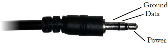
Figure 1: 3.5 mm Stereo Plug Wiring
