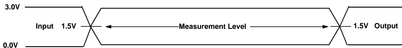
Figure 15. Input Waveforms and Measurement Levels
