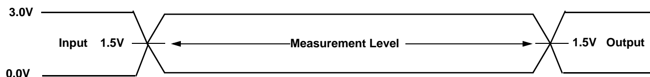
Figure 15. Input Waveforms and Measurement Levels
