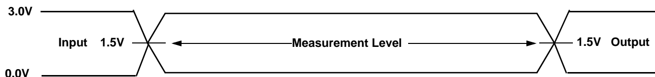
Figure 15. Input Waveforms and Measurement Levels
