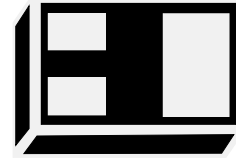
DFN1006-3L (Bottom View)
