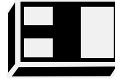
DFN1006-3L (Bottom View)
