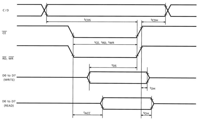
Test Conditions (Unless Otherwise Noted, VDD = 5.0 V ± 10%, VSS = 0 V, Ta = −20 to 75°C)
