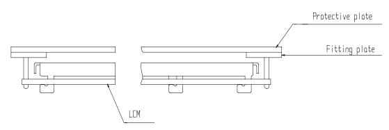
(2) When assembling the LCM into other equipment, the spacer to the bit between the LCM and the fitting plate should have enough height to avoid causing stress to the module surface, refer to the individual specifications for measurements. The measurement tolerance should be  $\pm 0.1$ mm.
