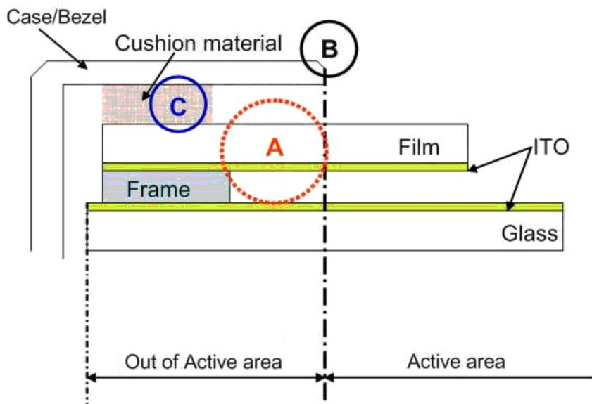
(vi) TO PREVENT GIVING DISTORTION TO THE FILM OF THE PRODUCT AND PEELING OFF OF THE FILM FROM THE PRODUCT, DO NOT FIX THE FILM AND A SET CASE OR A SHOCK ABSORBING MATERIAL ADHERED TO A SET CASE BY ADHESION.
