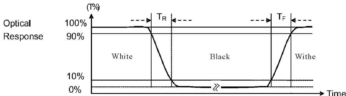
NOTE (5) : THE 100% TRANSMISSION IS DEFINED AS THE TRANSMISSION OF LCD PANEL WHEN ALL THE INPUT TERMINALS OF MODULE ARE ELECTRICALLY OPENED.
