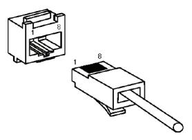
Figure 11: RJ45 Connector
