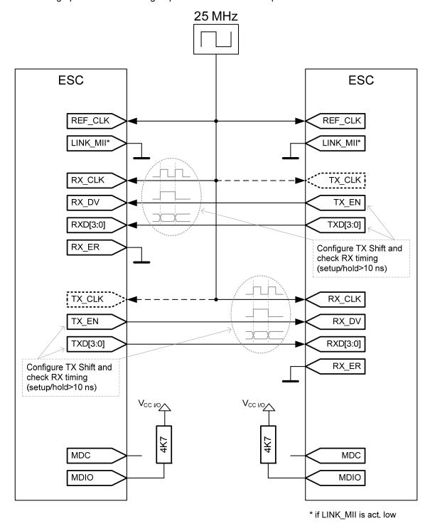
Figure 13: Back-to-Back Ethernet Connection
