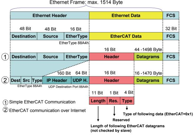
Figure 2: Ethernet Frame with EtherCAT Data
