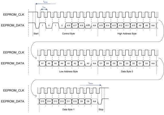
Figure 37: Write access (2 address bytes, 32 kBit - 4 MBit EEPROMs)
