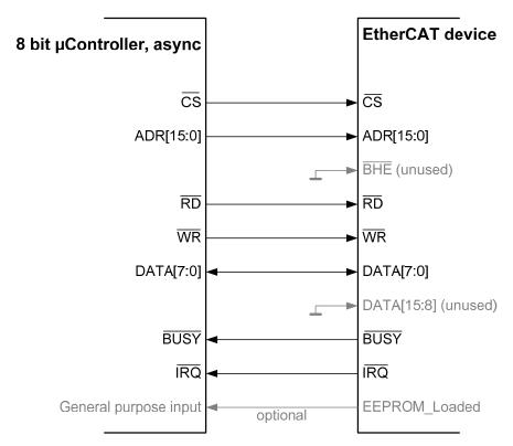
Figure 50: Connection with 8 bit µControllers (BHE and DATA[15:8] should not be left open)
