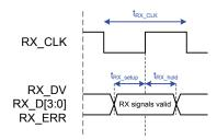
Figure 34: MII timing RX signals
