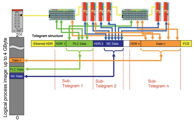
Figure 18: FMMU Mapping Principle
