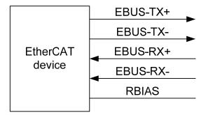
Figure 14: EBUS Interface Signals
