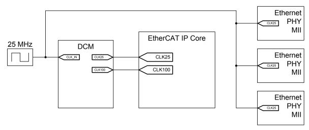
Figure 61: EtherCAT IP Core clock source (MII)
