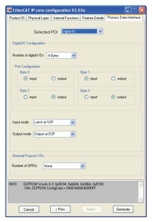
Figure 19: Register PDI - Digital I/O Configuration
