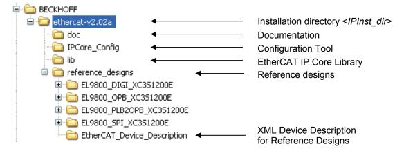
Figure 3: Files installed with EtherCAT IP core setup
