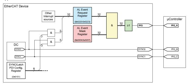
Figure 39: PDI Interrupt Masking and interrupt signals
