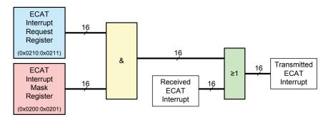
Figure 40: ECAT Interrupt Masking
