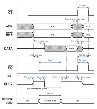
Figure 51: Read access (without preceding write access)
