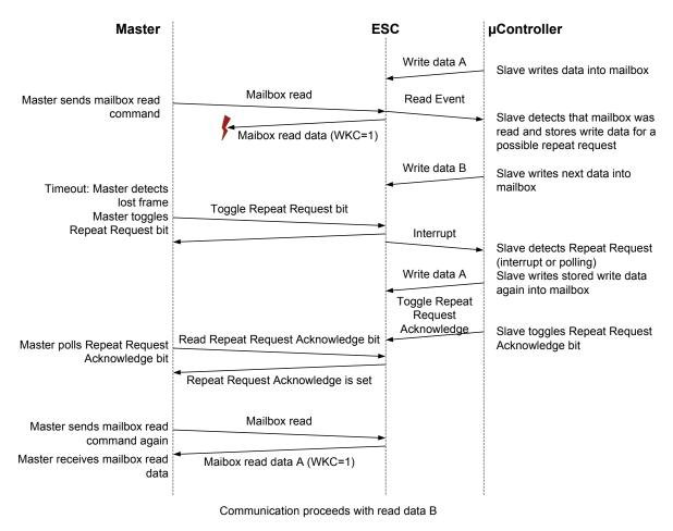
Figure 24: Handling of Write/Read Toggle with Read Mailbox
