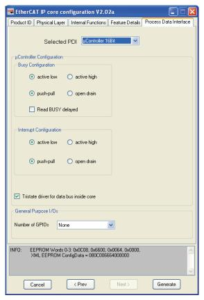
Figure 20: Register PDI - μC-Configuration
