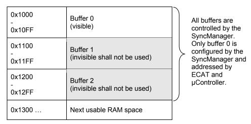
Figure 20: SyncManager Buffer allocation
