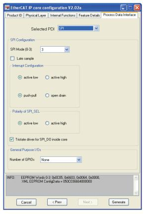
Figure 21: Register PDI - SPI Configuration
