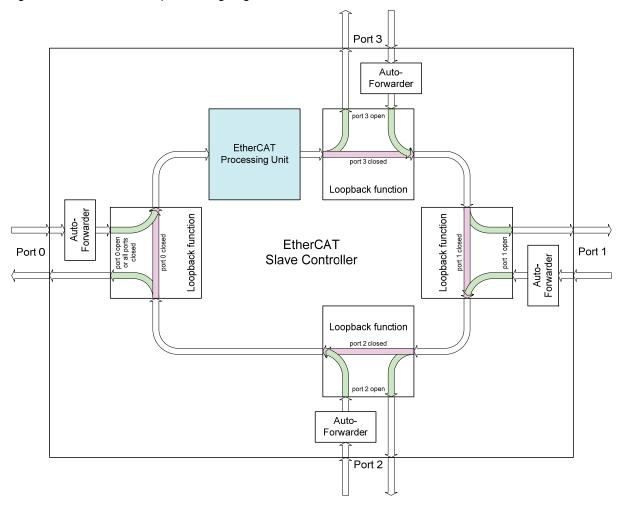
Figure 4: Frame Processing
