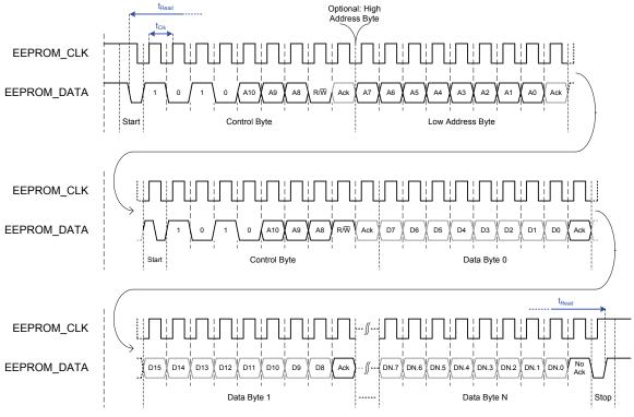
Figure 38: Read access (1 address byte, up to 16 kBit EEPROMs)
