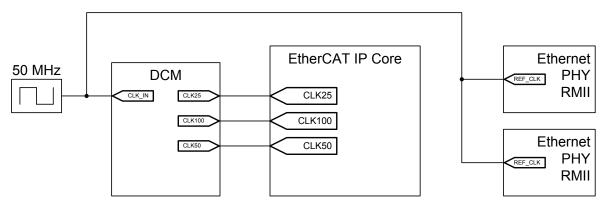
Figure 62: EtherCAT IP Core clock source (RMII)
