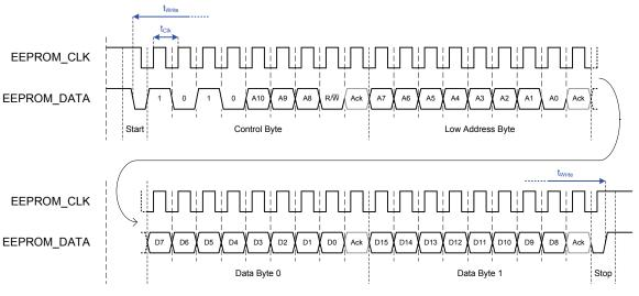
Figure 36: Write access (1 address byte, up to 16 kBit EEPROMs)
