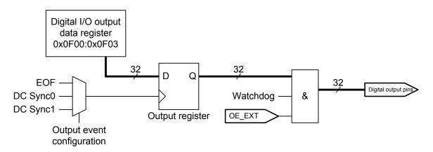
Figure 37: Digital Output Principle Schematic
