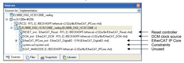
Figure 7: ISE Sources Window - FPGA designs
