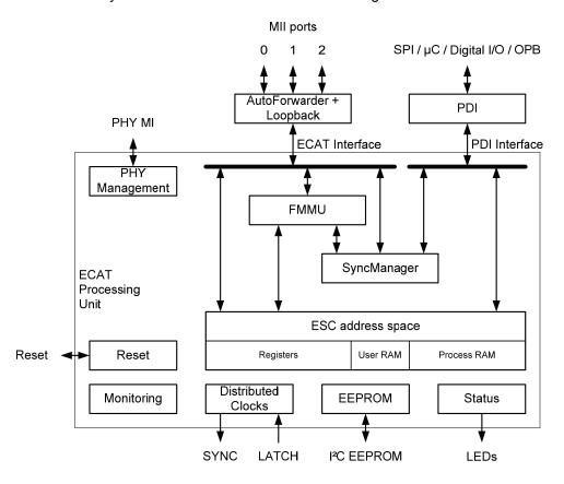
Figure 1: EtherCAT IP Core Block Diagram
