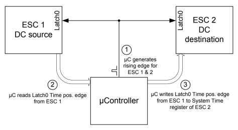
Figure 30: System Time PDI Controlled with three steps
