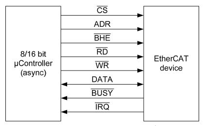
Figure 48: µController interconnection<sup>8</sup>
