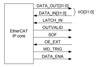
Figure 36: IP core digital I/O signals
