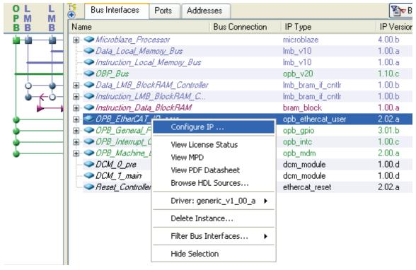
Figure 26: EDK - Configuration of IP Core
