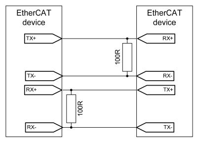
Figure 17: EBUS Connection
