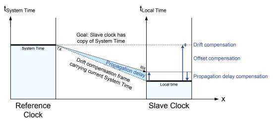
Figure 25: Propagation Delay, Offset, and Drift Compensation
