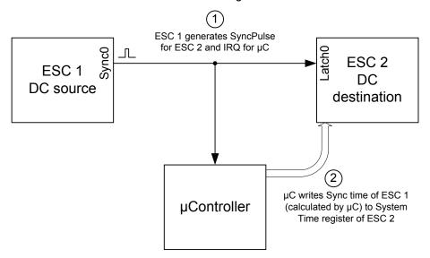
Figure 31: System Time PDI Controlled with two steps
