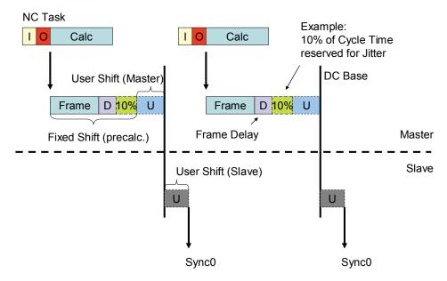
Figure 32: DC Timing Signals in relation to Communication
