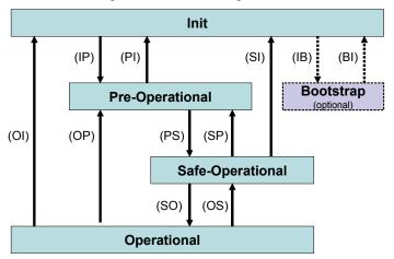
Figure 33: EtherCAT State Machine
