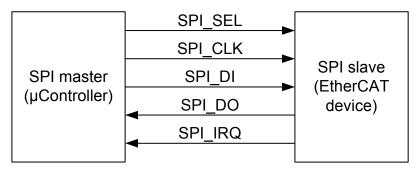
Figure 42: SPI master and slave interconnection
