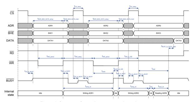
Figure 53: Sequence of two write accesses and a read access
