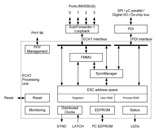
Figure 1: EtherCAT Slave Controller Block Diagram
