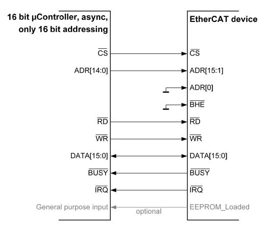
Figure 49: Connection with 16 bit µControllers without byte addressing
