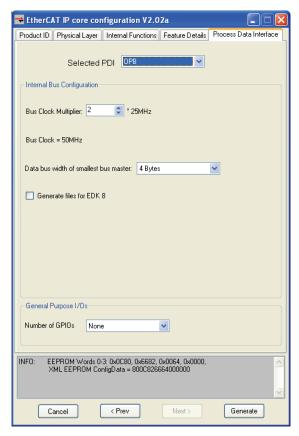
Figure 22: Register PDI - OPB Interface Configuration
