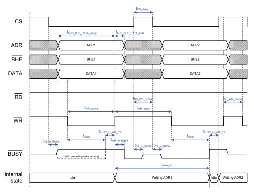
Figure 52: Write access (without preceding write access)
