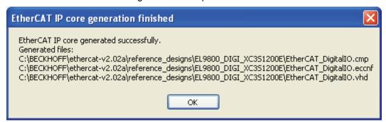
Figure 6: IP Core generation successful
