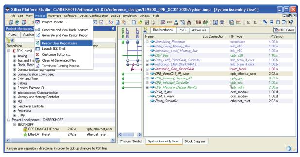
Figure 25: EDK - Rescan Repository after changing IP Core Configuration
