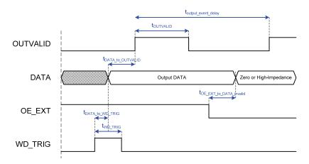
Figure 40: Digital Output timing
