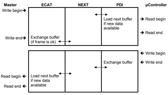
Figure 21: SyncManager Buffered Mode Interaction
