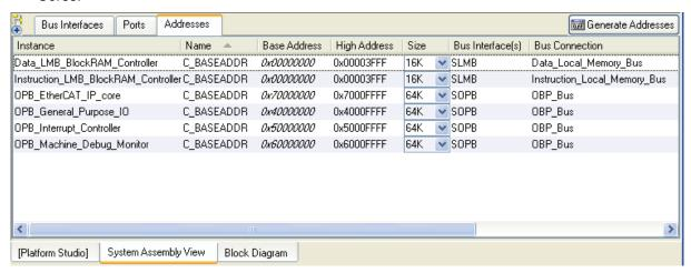
Figure 28: EDK - System Assembly View, Filter Addresses
