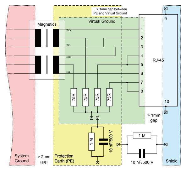
Figure 10: Termination and Grounding Recommendation
