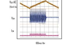
Light load Switching Waveform
