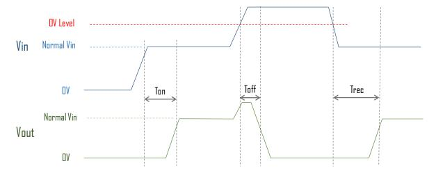
Ton : the time from 90% Vin at VIN termianl to 90% Vin at VOUT terminal
