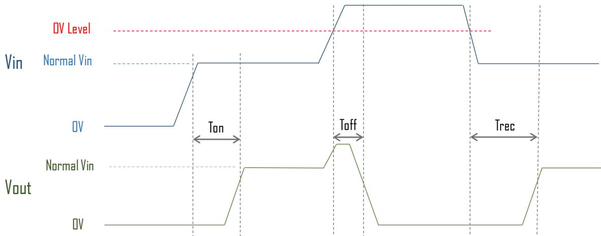
$T_{on}$  : the time from 90%  $V_{in}$  at  $V_{IN}$  terminal to 90%  $V_{in}$  at  $V_{OUT}$  terminal
