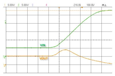
Recovery delay time Vin drop from 30V to 5V Trec = 250us
