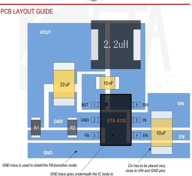
$R_1 = \left(\frac{V_{OUT}}{V_{REF}} - 1\right) \times R_2$
