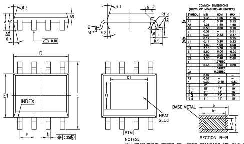
NOTES: SECTION B-B ALL DIMENSIONS REFER TO JEDEC STANDARD MS-012 AA DO NOT INCLUDE MOLD FLASH OR PROTRUSIONS.
