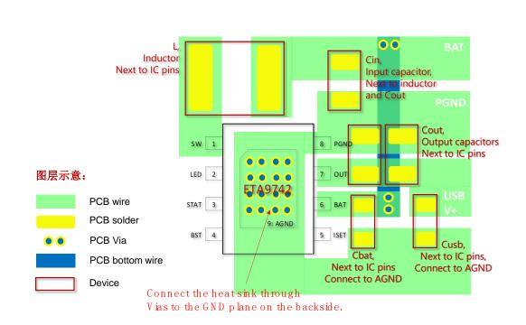
Please have CIN, COUT, and L placed just next to the IC pins so that the power traces are kept to the shortest to achieve a good performance of ETA9742 and good EMI.
