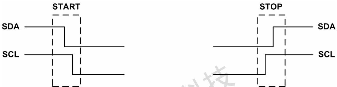
Figure 4. I 2 C STOP and START Conditions
