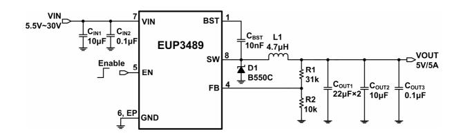
**Figure 1. 5V Application Circuit**
