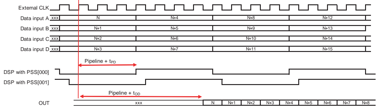
Figure 3-1. Timing Diagram for 4:1 MUX principle of operation OCDS1, IUCM1
