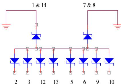
The EiMDXXC8 is designed to provide transient suppression on multiple data lines and I/O ports. The low profile SO-14 design allows the user to protect up to eight data and I/O lines with one package. The bidirectional device and may be used on lines where the normal operating voltage is above and below ground (i.e. +12V to -12V). The EiMDXXC8 TVS diode network will meet the surge requirements of IEC 1000-4-2, Level 4, "Human Body Model" for air and contact discharge.
