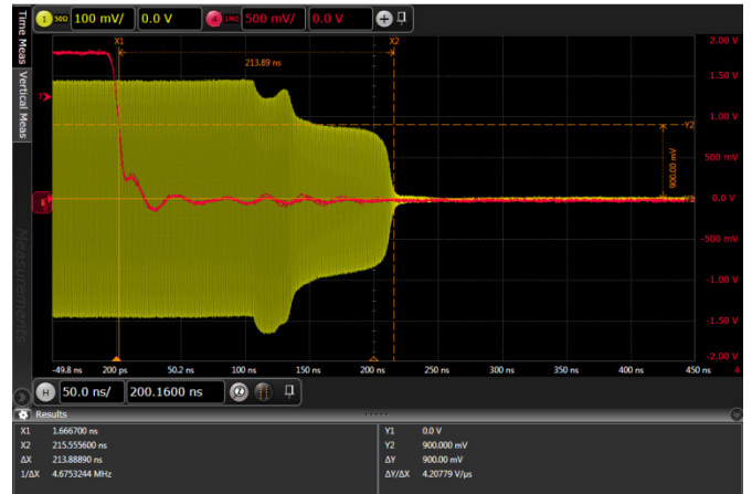
Figure 17. Switching Time Insertion Loss to Isolation
