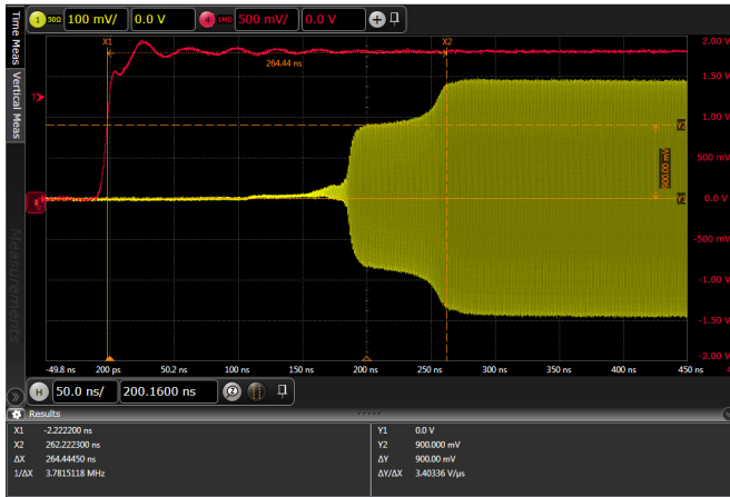
Figure 16. Switching Time Isolation to Insertion loss
