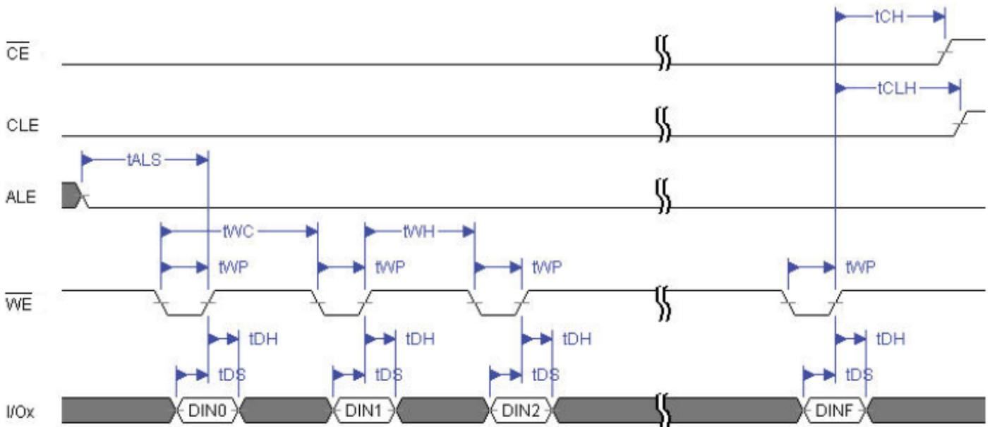
**Serial access Cycle after Read (CLE = L, ALE = L,  $\overline{WE}$  = H)**
