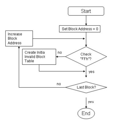
Check "FFh" at the 1st Byte column address in the spare area of the 1st and 2nd page in the block.
