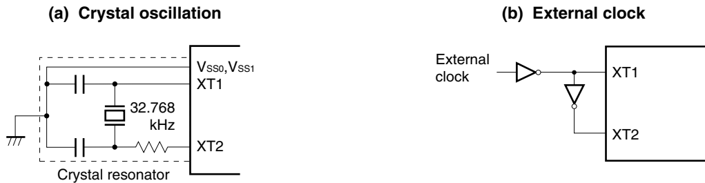
Figure 5-6. External Circuit of Subsystem Clock Oscillator
