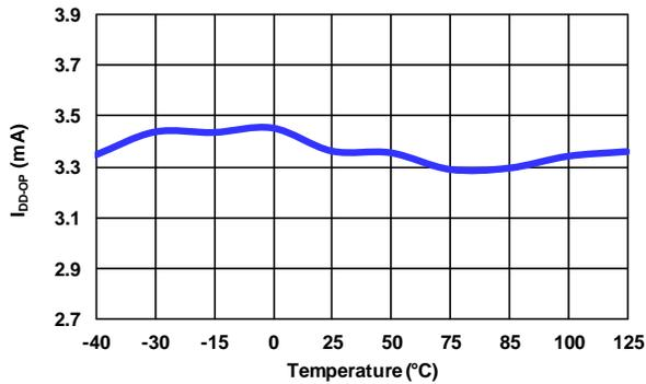
Figure 8. Operating Supply Current (I<sub>DD-OP</sub>) vs. Temperature
