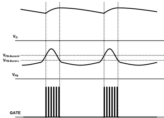
Figure 29. Burst-Mode Operation
