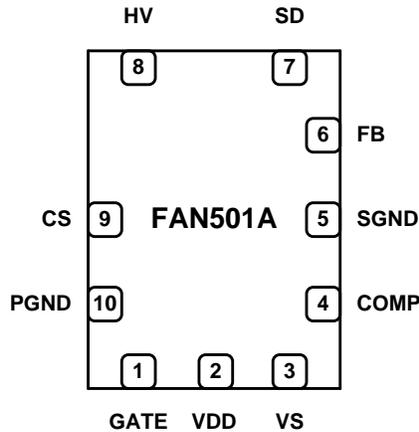
Figure 5. Pin Assignments
