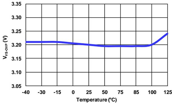
**Figure 12. Output OVP with V<sub>S</sub> Sampling Voltage (V<sub>VS-OVP</sub>) vs. Temperature**
