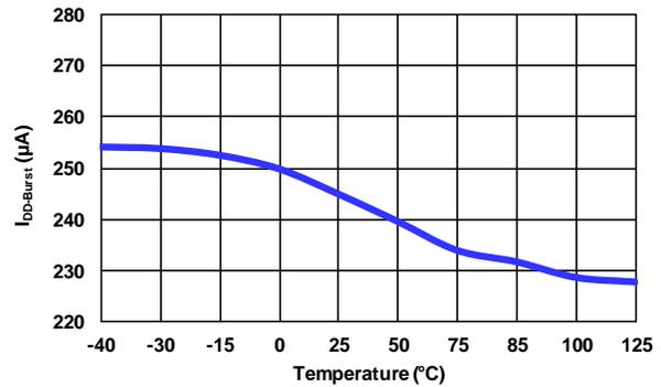
Figure 9. Burst Mode Operating Supply Current (I<sub>DD-Burst</sub>) vs. Temperature
