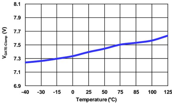
**Figure 18. Gate Output Clamping Voltage (V<sub>GATE-Clamp</sub>) vs. Temperature**
