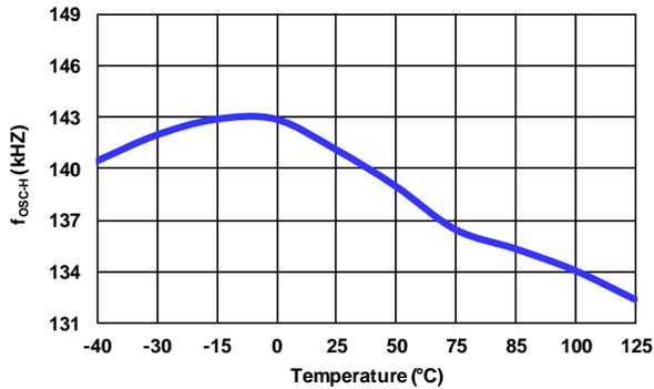
Figure 10. Operating Frequency, I<sub>VS</sub> < I<sub>VS-L</sub> Threshold (f<sub>OSC-H</sub>) vs. Temperature
