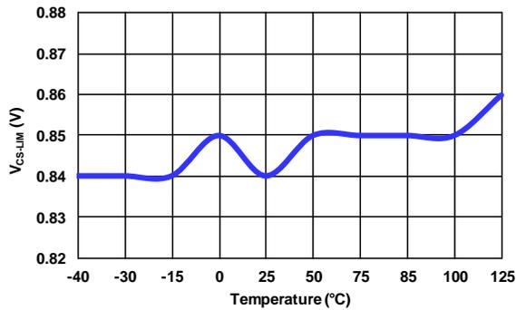
**Figure 16. Current Limit Threshold Voltage (V<sub>CS-LIM</sub>) vs. Temperature**
