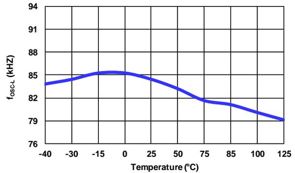
Figure 11. Operating Frequency while I<sub>VS</sub> < I<sub>VS-H</sub> Threshold (f<sub>OSC-L</sub>) vs. Temperature
