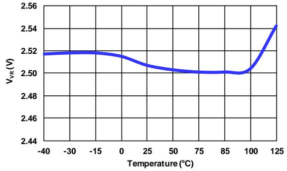
**Figure 13. Internal Reference Voltage for CC Regulation (V<sub>VR</sub>) vs. Temperature**
