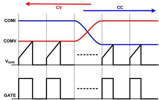
Figure 20. PWM Operation for CV / CC Regulation
