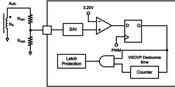
Figure 34. V<sub>S</sub> OVP Protection Circuit
