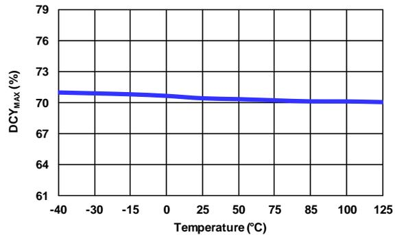
**Figure 17. Maximum Duty Cycle (DCY<sub>MAX</sub>) vs. Temperature**
