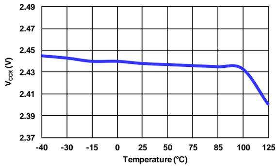
**Figure 14. Variation Test Voltage on CS Pin for CC Regulation (V<sub>CCR</sub>) vs. Temperature**
