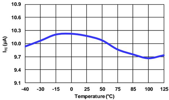
**Figure 15. Temperature-Independent Bias Current (I<sub>TC</sub>) vs. Temperature**
