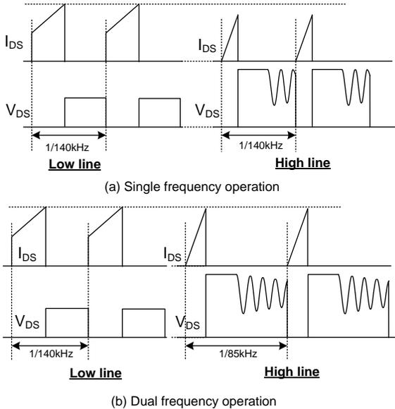
**Figure 24. Peak Switch Current, Single- and Dual-Frequency Operation**
