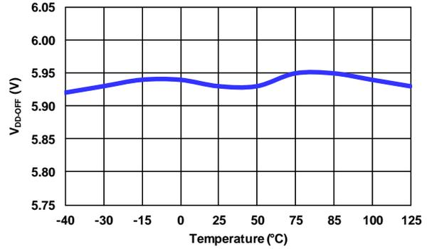
Figure 7. V<sub>DD</sub> Turn-Off Threshold Voltage (V<sub>DD-OFF</sub>) vs. Temperature
