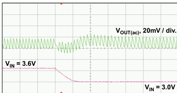
Figure 28. Line Transient, 600mV, 50mA Load
