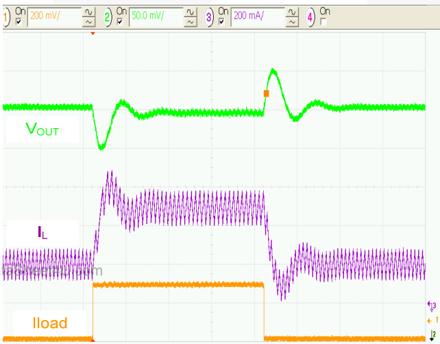
Figure 15. Load Transient 200 to 500mA, 3.6V IN , 5μs/div.
