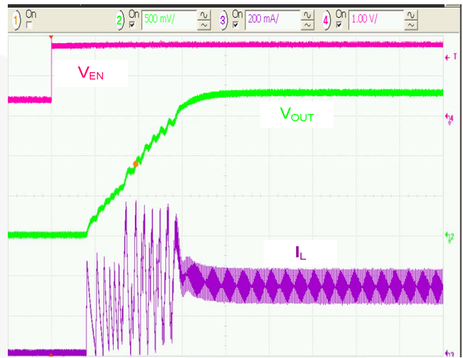
Figure 18. Soft-Start, R_{LOAD} = 6\Omega , 20 \mu s/div.
