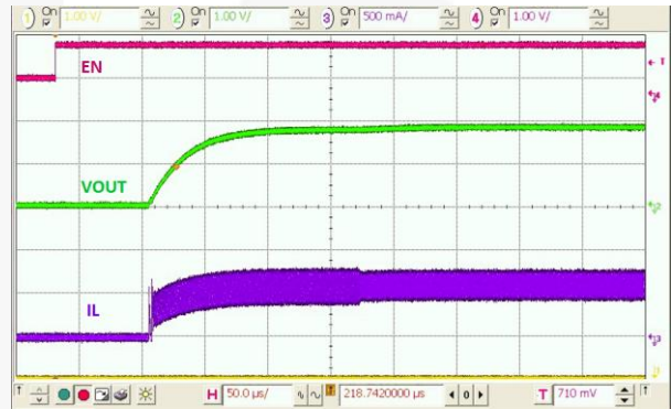
Figure 25. Startup, 3 \Omega Load
