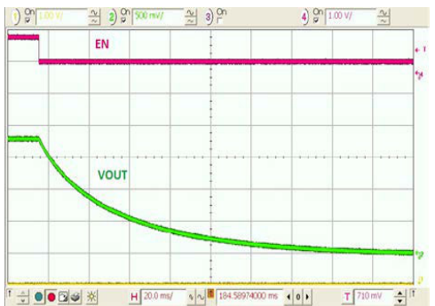
Figure 26. Shutdown, 10 \text{k}\Omega Load, No Output Discharge
